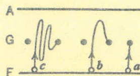
Fig. 6. Barkhausen Kurz U.H.F. Oscillator. The circuit is similar to Fig. 1, but the plate anode is run at a lower voltage than the grid.
